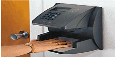
Access Control Terminal
